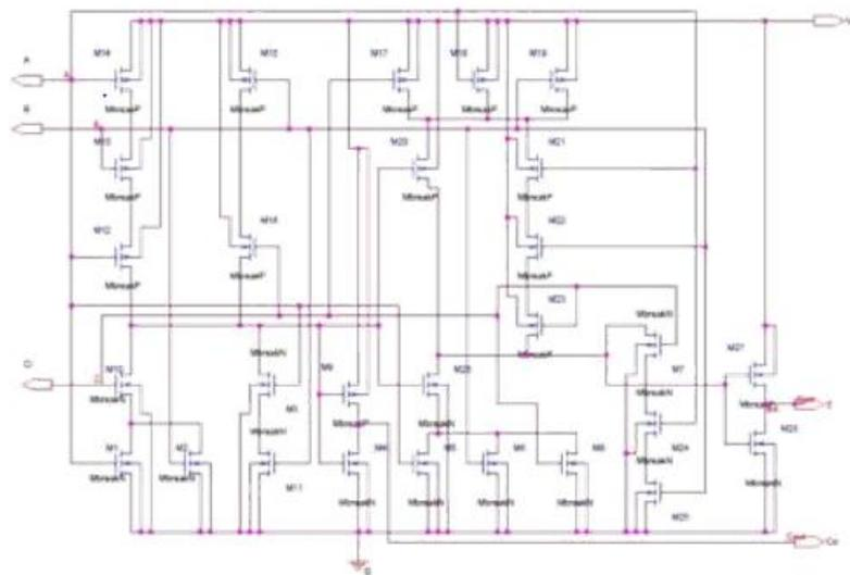
Fig. 3: Schematic structure of ALU transistor model
