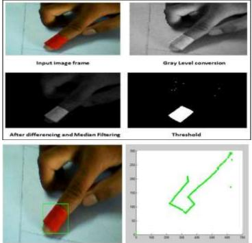
Fig.12. MATLAB simulation for moving object tracking
