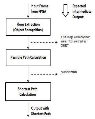
Fig.9. Flowchart of Path calculation algorithm
