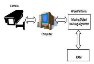
Fig.2: Layout of the Image Processing System
