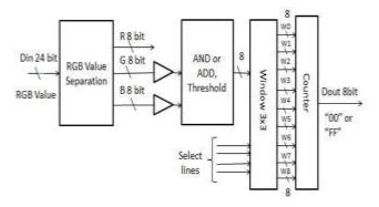
Fig. 5. Architecture of proposed FPGA module
