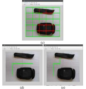
**Fig.11.** Path finding results (a) Original image (b) Floor extracted image (c) Possible movable paths shown in green (d) (e) shortest path output with two different destination coordinate
