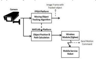
Fig. 1: System Block Diagram
