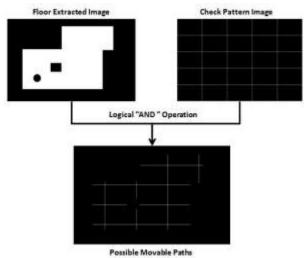
Fig.10. Chessboard pattern method; white area in first image floor area.
