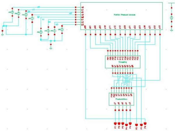
Fig. 7 A 4x4 bit reduced complexity wallace multiplier
