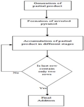
Fig. 6 Flowchart for designing a reduced complexity wallace multiplier
