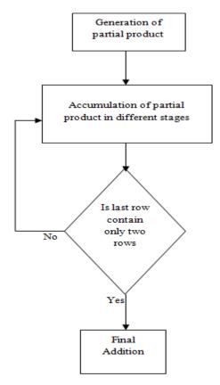
Fig. 2 Flowchart for designing a conventional wallace multiplier
