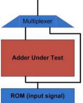
Fig. 3. Circuit used to test the adders
