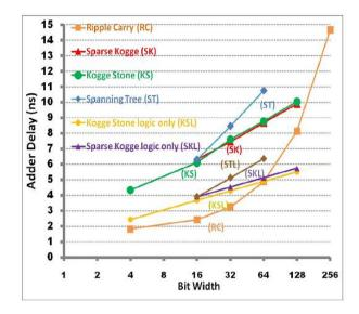
Fig. 6. Simulation results for the adder designs
