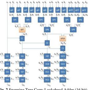
Fig. 2.Spanning Tree Carry Lookahead Adder (16 bit)
