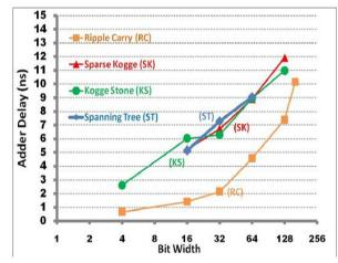
Fig. 7. Measured results for the parallel-prefix adder designs compared with the RCA.
