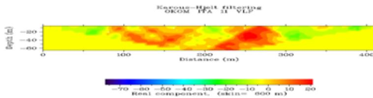
Fig. 36: Current density cross section plot of in-phase data against distance at location VLF 11
