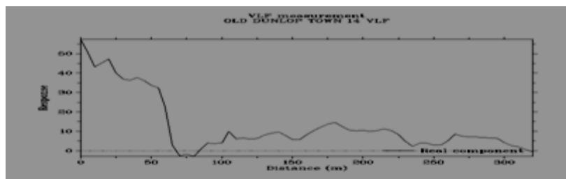
Fig. 43: A plot of unfiltered in-phase data against distance at location VLF 14
