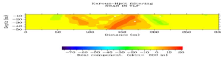
Fig. 57: Current density cross section plot of in-phase data against distances at location VLF 18
