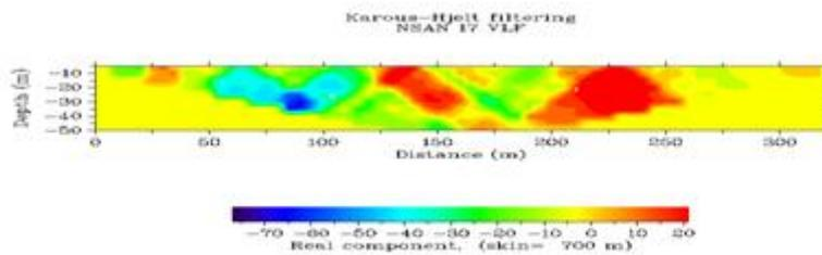
Fig.54: Current density cross section plot of in-phase data against distances at location VLF 17
