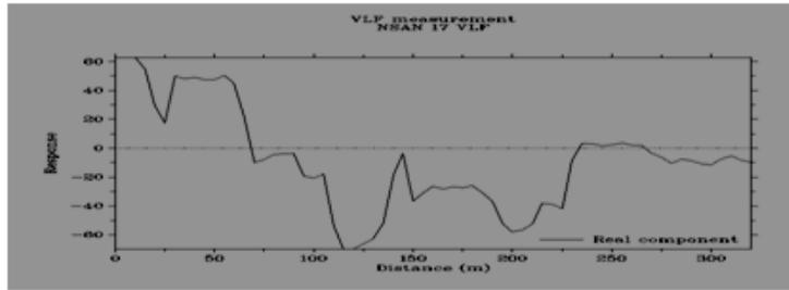
Fig. 52: A plot of unfiltered in-phase data against distance at location VLF 17
