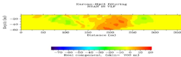
Fig. 51: Current density cross section plot of in-phase data against distance at location VLF 16
