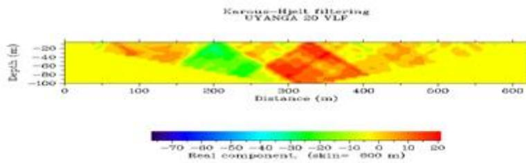
Fig. 63: Current density cross section plot of in-phase data against distances at location VLF 20
