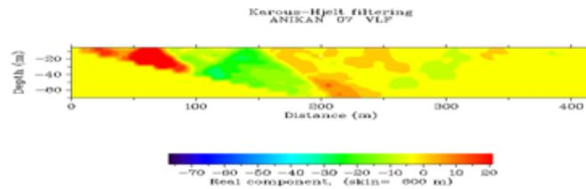
Fig. 24: Current density cross section plot of in-phase data against distance at location VLF 07
