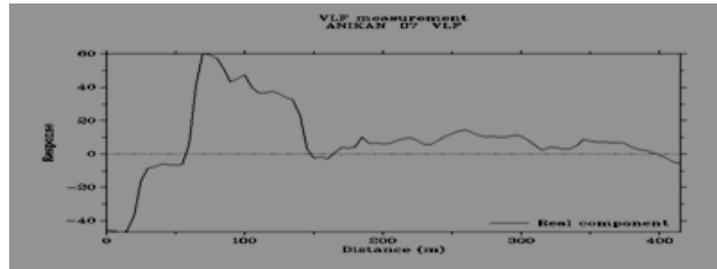
Fig. 22: A plot of unfiltered in-phase data against distance at location VLF 07
