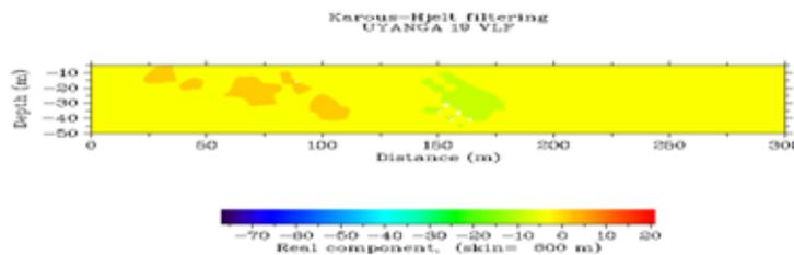
Fig. 59: Current density cross section plot of in-phase data against distances at location VLF 19
