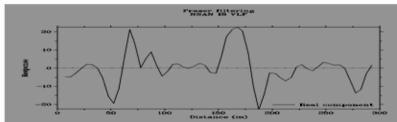
Fig. 56: A plot of filtered in-phase data against distance at location VLF 18
