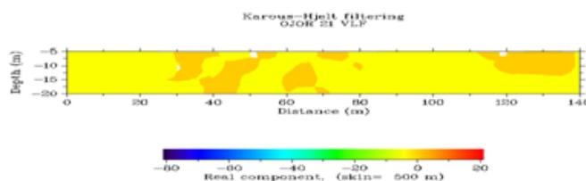
Fig. 66: Current density cross section plot of in-phase data against distances at location VLF 21
