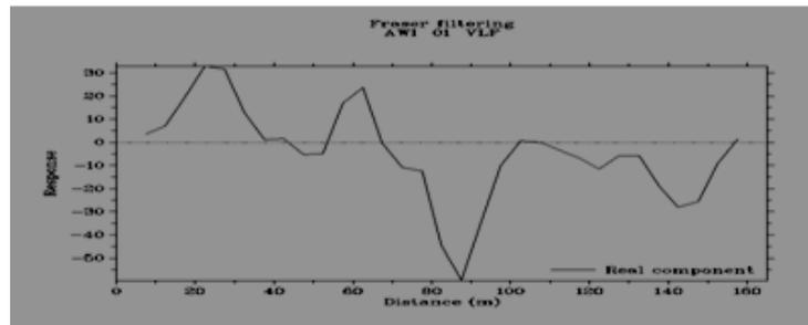
Fig. 5: A plot of filtered in-phase data against distance at location VLF 01
