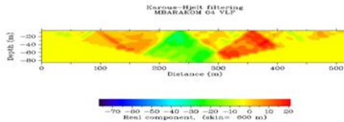
Fig.15: Current density cross section plot of in-phase data against distance at location VLF 04
