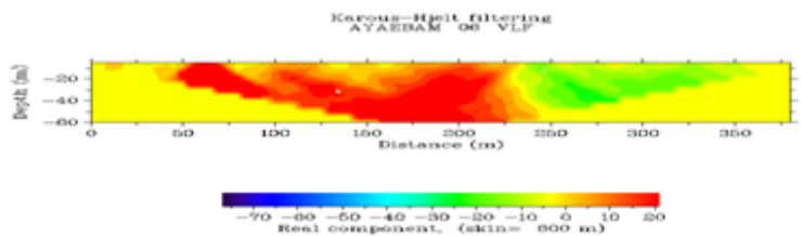
Fig. 21: Current density cross section plot of in-phase data against distance at location VLF 06
