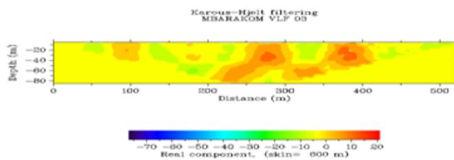
Fig. 12: Current density cross section plot of in-phase data against distance at location VLF 03
