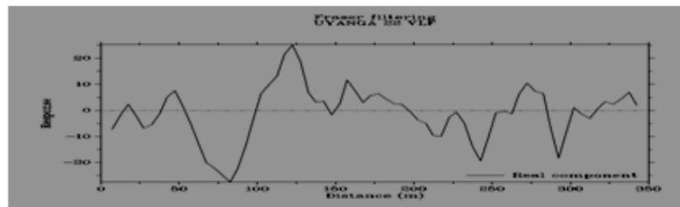
Fig. 68: A plot of filtered in-phase data against distance at location VLF 22
