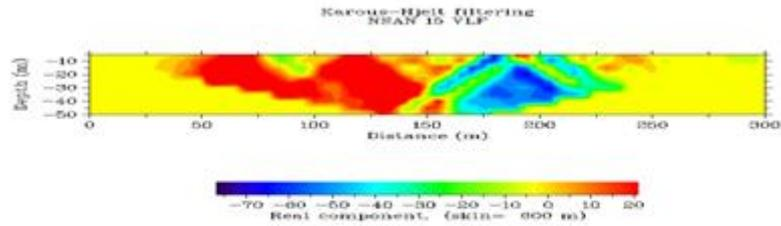
Fig. 48: Current density cross section plot of in-phase data against distance at location VLF 15
