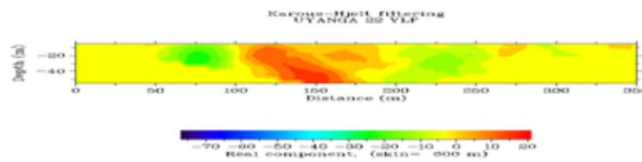
Fig. 69: Current density cross section plot of in-phase data against distances at location VLF 22
