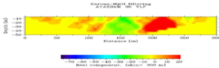
Fig.18: Current density cross section plot of in-phase data against distance at location VLF 05
