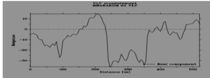
Fig. 13: A plot of unfiltered in-phase data against distance at location VLF 04
