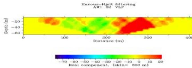
Fig. 9: Current density cross section plot of in-phase data against distance at location VLF 02
