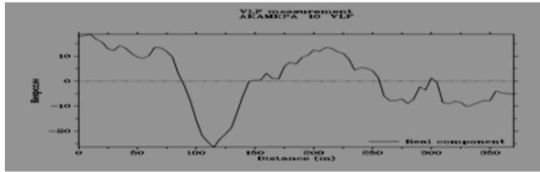
Fig. 31: A plot of unfiltered in-phase data against distance at location VLF 10
