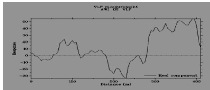
Fig. 7: A plot of unfiltered in-phase data against distance at location VLF 02
