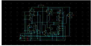
Fig.(e) Schematic View of 28T Adder Circuit
