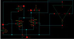
Fig.(w) Schematic of transmission gate
