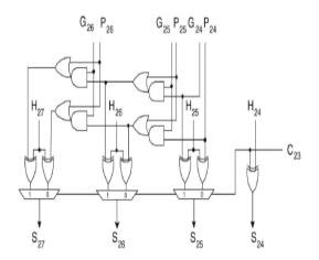
Fig.3. Logic-level implementation of a 4-bit carry-select block
