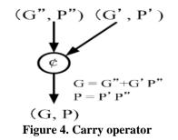
A parallel prefix adder can be represented as a parallel prefix graph consisting of carry operator nodes. Figure 5 is the parallel prefix graph of a Ladner-Fischer adder. This adder structure has minimum logic depth, but has large fan-out requirement up to n/2.
