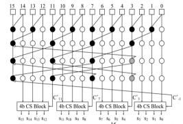
Fig. 7.Proposed sparse-4 modulo  $2^{16} + 1$  diminished-1 adder.
