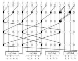
Fig 6 Modulo 2<sup>16</sup>+1 diminished adders using a sparse carry computation unit.
