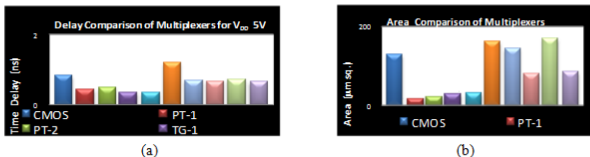
Figure 27: (a) Delay Comparison of Multiplexers for V DD 5V (b) Area Comparison of Multiplexers
