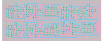
Figure 14 layout of 2-bit Sklansky adder
