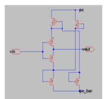
Figure2: CEPAL inverter schematic
