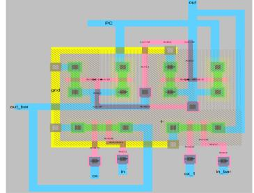
Figure6 CAL inverter layout
