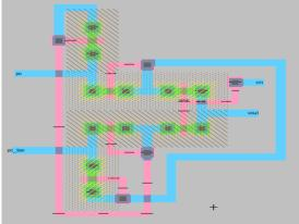
Figure3 CEPAL inverter layout
