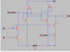
Figure5 CAL inverter schematic
