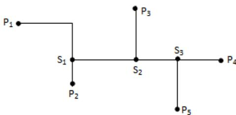
Fig. 1 Rectilinear Steiner Minimum Tree
