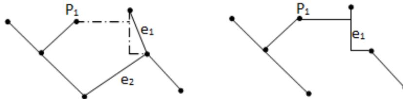
Fig. 5 Edge based heuristic
