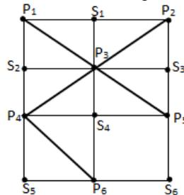
Fig. 4 MST over P and the Candidate Steiner Points (CSPs)
