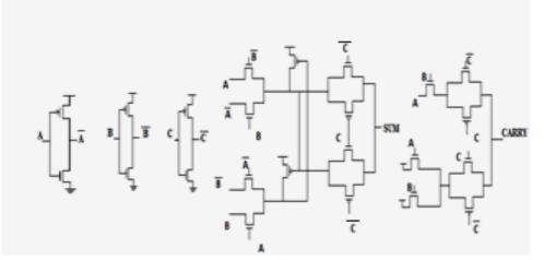
Figure 4: Full-adder designed with the Proposed Logic structure and a Pass Transistor Logic Style
