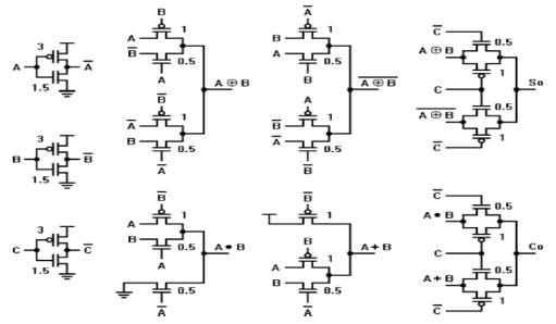
Figure 2: Full-adder designed with the Existing logic Structure and a DPL Logic Style.
