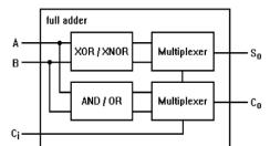
Figure 1: Alternative logic scheme for designing full-adder cells. Table 1
