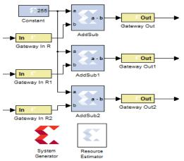
Figure 7: Algorithm for Color Image Negative using Addsub Block
