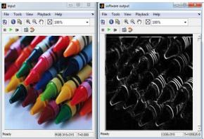
Figure 21: Results for Sobel X-Y detection Grayscale.
