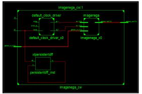
Figure 27: RTL Schematic for Image Negative
