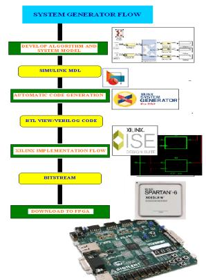
Figure 1: Design flow for Xilinx System Generator
