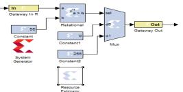
Figure 18: Algorithm for image Thresholding
