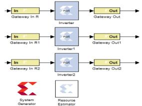
Figure 8: Algorithm for Color Image Negative using Inverter Block
