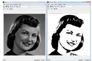
Figure 19: Results for thresholding
