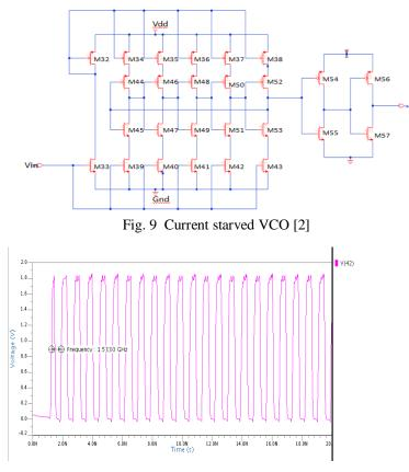
Fig. 10 Simulation result of VCO at 90mV input voltage
