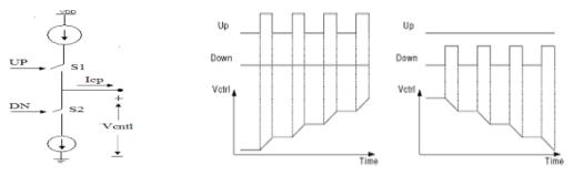
Fig 2 Basic block diagram of Charge Pump with Ideal Behavior [1]
