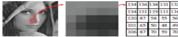
(a) original image (b) Region of red rectangle (c) Gray-scale value Fig. 4. A non-smooth region in Lena
