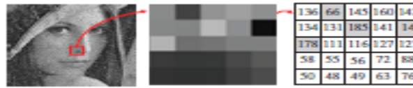
(a) original image (b) Region of red rectangle (c) Gray-scale value Fig. 5. The difference between noisy and neighboring pixels in Lena
