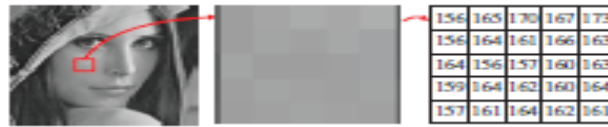
(a) original image (b) Region of red rectangle (c) Gray-scale value Fig. 3. A smooth region in Lena
