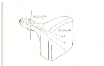
Fig 9 electron motion in CRO
