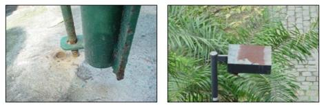
Figures 15, 16 – Atmospheric corrosion of rod and box of carbon steel.
