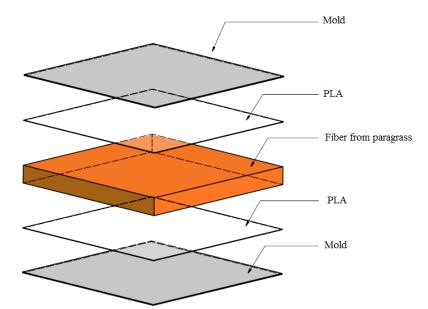
Fig. 1 Preparation of composite from PLA and paragrass fiber by laminated technique
