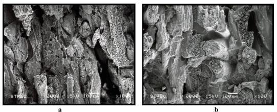
Fig. 7 Morphological study of composite prepared from PLA/fiber (a) Paragrass fiber/PLA composites (b) Silane treated Paragrass fiber/PLA composites
