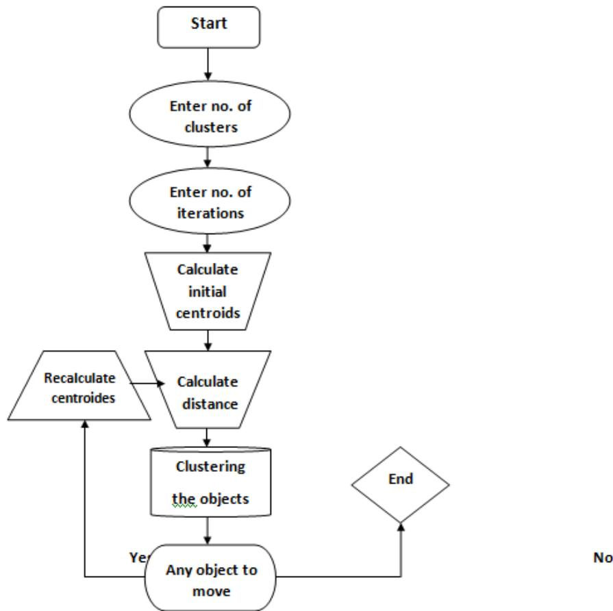
Figure 2. Flow chart of the K-means algorithm.
