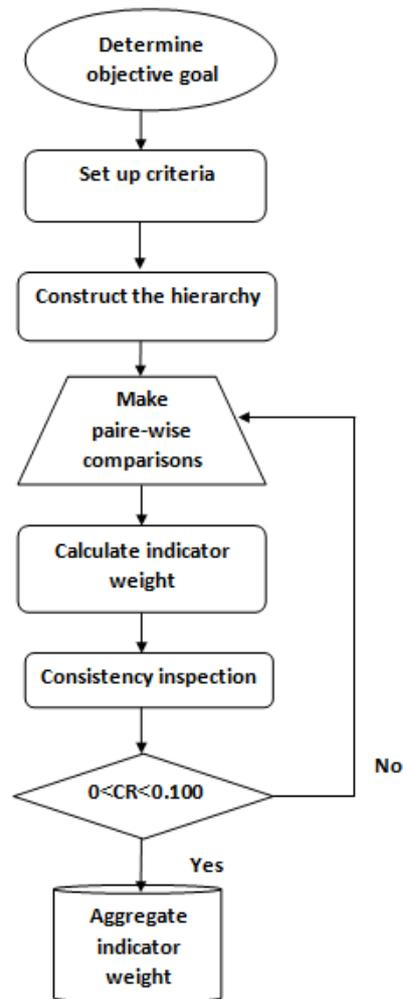
**Figure 1.**Flow chart of the AHP algorithm.
