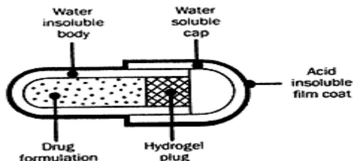
**Fig.1: Design of Flurbiprofen pulsatile capsule device**
