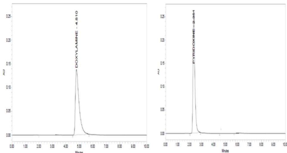
**Fig. No. 2** Chromatogram showing assay injection of PYR and DOX.
