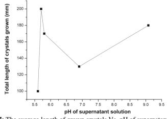
Figure 7: The average length of grown crystals Vs. pH of supernatant solution
