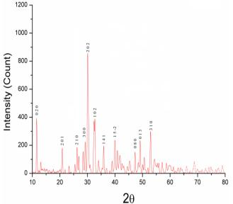
Figure 3: XRD pattern of brushite crystals
