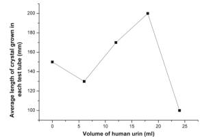
Figure 6: The plot of average length of grown brushite crystals Vs. volume of human urine.
