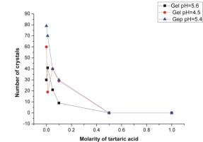
Figure 8: The number of brushite crystals grown Vs. the molar concentration of tartaric acid for different pH values
