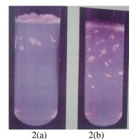
Figure 2(a, b): CHPD crystal growth in the presence of 8 ml and 16 ml human urine in the supernatant solution
