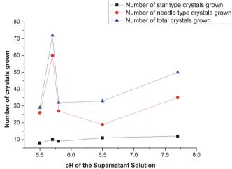
Figure 5: Number of crystals grown Vs. pH of supernatant solution
