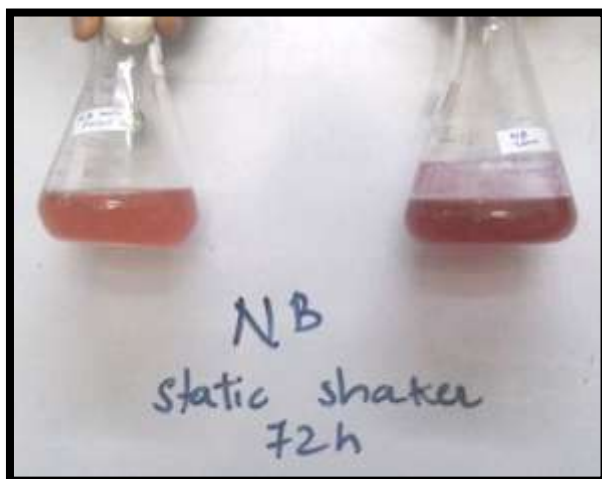
Figure 5.3.4. Effect of static/shaker conditions on prodigiosin production
