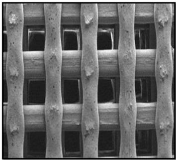
Fig.11.showing the SEM image of scaffold prepared by rapid prototype technique
