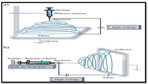
Fig.5. Schematic diagram of Electrospinning fabrication technique
