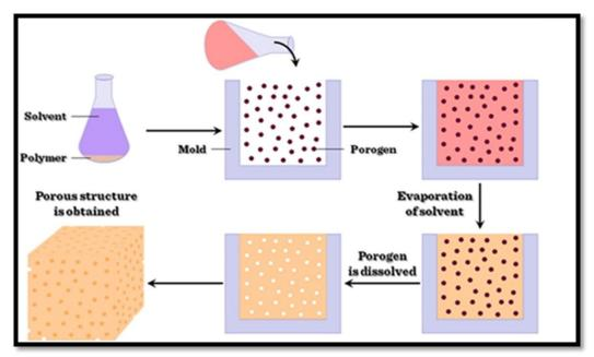
Fig 4. Schematic diagram of Solvent casting-particulate leaching scaffold fabrication technique.
