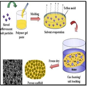
Fig.7.Schematic diagram of Gas-Foaming Scaffold fabrication Technique
