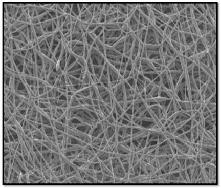
Fig 6. SEM image of scaffold prepared by Electrospinning technique
