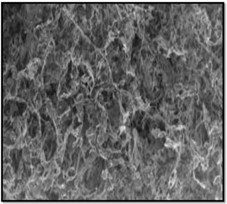
Fig. 8.SEM image of scaffold prepared by Gas-Foaming Process.
