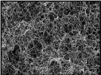
Fig.12. Showing SEM image of scaffold prepared by thermally induced phase separation.
