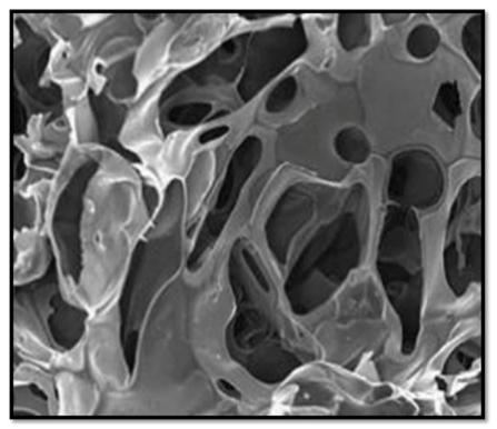
Fig.9.SEM image of scaffold prepared by emulsion-freeze drying process
