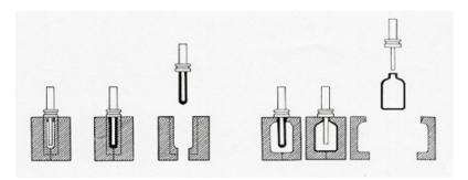
Injection blow molding include the following steps: at first, the polymer is injection molded onto the core pin; then the core pin is rotated to a blow molding station to be inflated and cooled.
