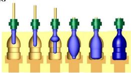
For Stretch Blow Molding, the polymer is first heated to aboe the glass transition temperature. Then polymer is inflated and stretched with a hollow core-rod. This process resembles that of a rubber balloon inflation.
