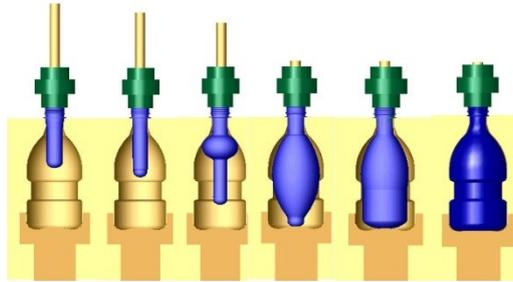
For Stretch Blow Molding, the polymer is first heated to above the glass transition temperature. Then polymer is inflated and stretched with a hollow core-rod. This process resembles that of a rubber balloon inflation.
