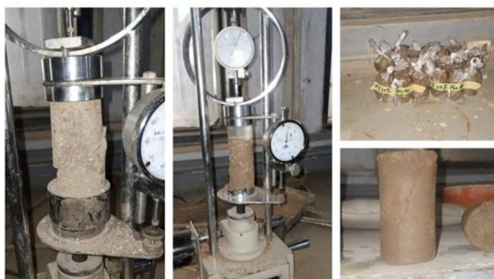
Fig. 4. UCS Tests in Progress
