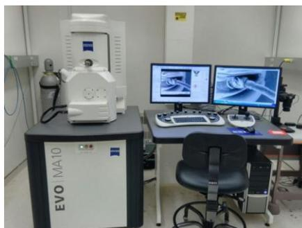
Figure 3. Scanning Electron Microscope (SEM)
