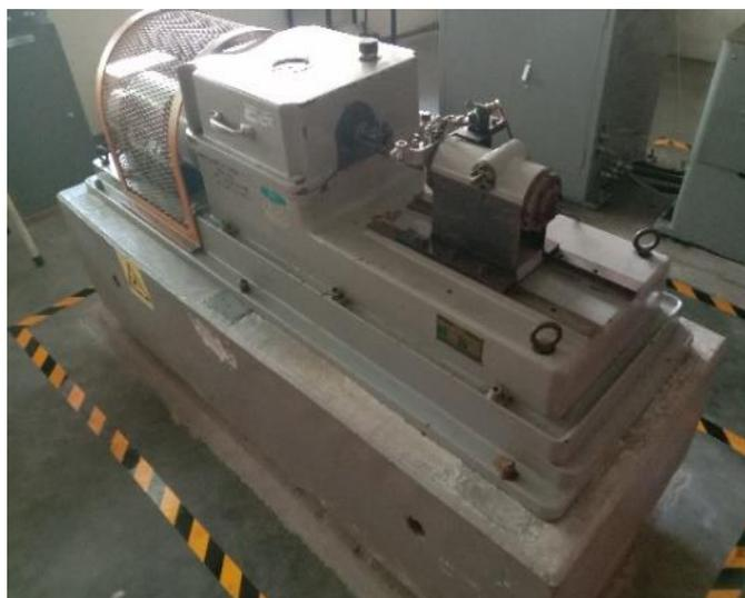
**Figure 2. Repeated Torsion and Bending Fatigue Testing Machine**
