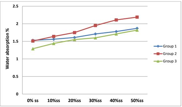
Fig.6. Concrete mixes water absorption after 28 days
