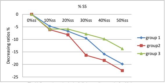
Fig.11. Decreasing ratios in the Splitting tensile strength after 28 days
