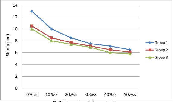
Fig.3. Slump values of all concrete mixes
