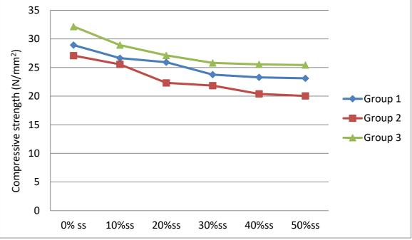
Fig. 8 Compressive strength of all concrete mixes after 28 days
