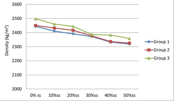
**Fig.4.** Density of all concrete mixes after 28 days
