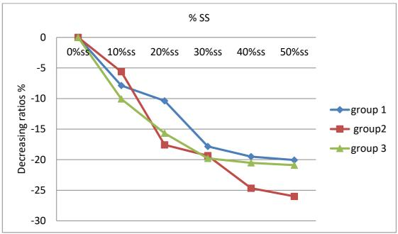
Fig.9 Decreasing ratios in the compressive strength after 28 days
