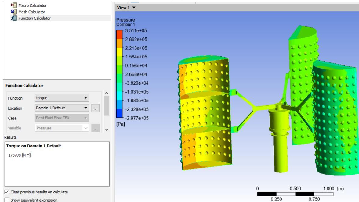
Fig. 6. Savonius wind turbine simulates CFD model with dimples and fins
