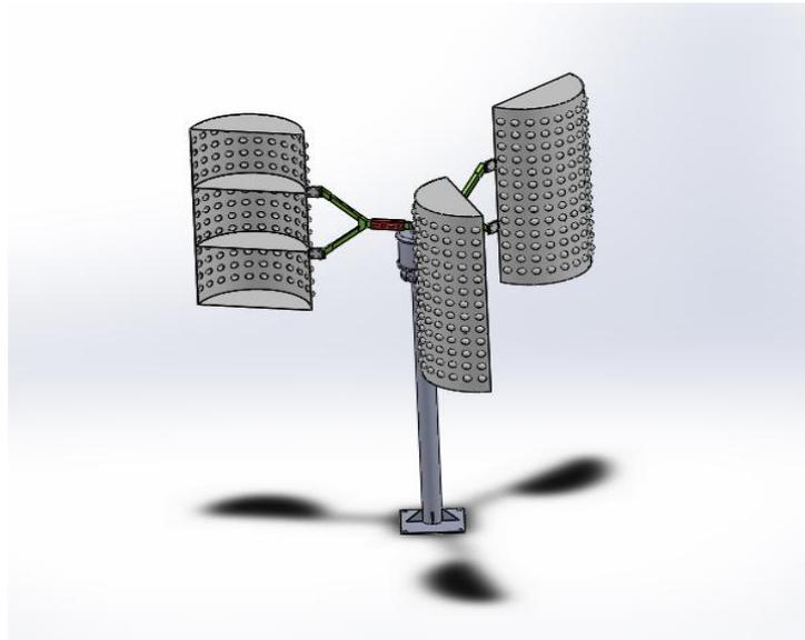
Fig. 3. Savonius VAWT with dimples and fins
