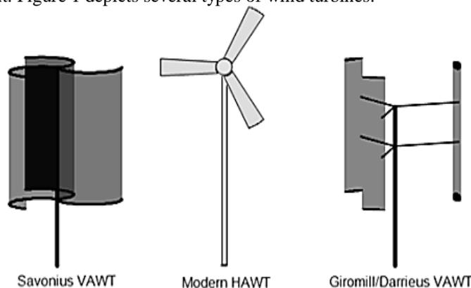
Fig. 1. Types of wind turbines
