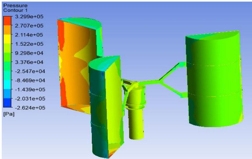
Fig. 5. Pressure contour on the blade of SAVTs without Dimples and fins
