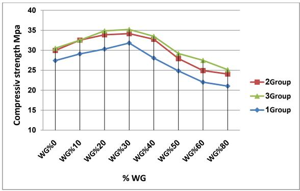
Figure [4] Variation of Compressive strength [[MPa]]
