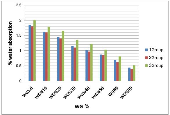
Figure [3] Values of water absorption
