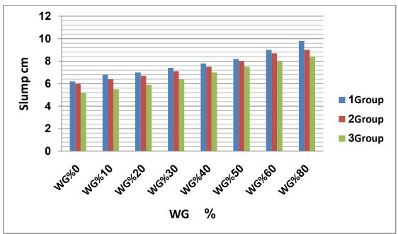
Figure [1] Values of the slump [cm]
