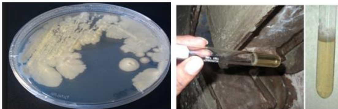
Fig.2: (a) Formation of Bacteria on agar plate (b) Bacteria before mixing to the concrete
