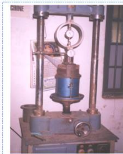
Fig.4 California Bearing Ratio Test Apparatus
