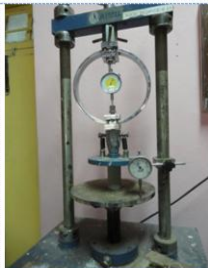
Fig.5 Unconfined Compressive Testing Machine
