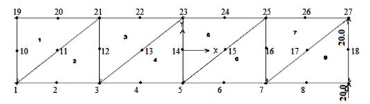
Fig. 4.1 FE Model for Test Example 1 – Cantilever Beam.
