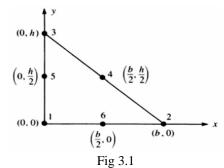
Fig 3.1 The triangle has a base dimension of b and a height h, with midside nodes. The general form of the displacement expressions in terms of the interpolation functions is given as
