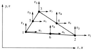
**Fig. 2.2:** Linear Strain Triangle (LST)
