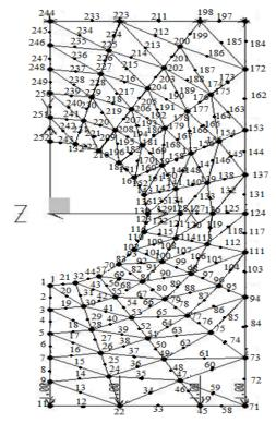
Fig. 7.3 FE Model for Test Example 3 – Plate with Semi Circular Hole.
