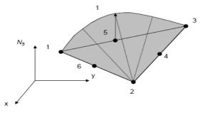
Fig 3.3: Interpolation function N<sub>5</sub>
