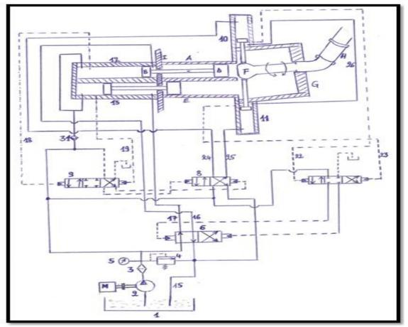
The bellow circuit combines together all mechanical parts and hydraulic parts. And shows how this automobile concrete pump works
