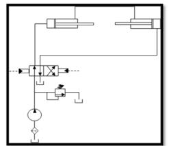
Figure 4: Hydraulic circuit commands swing tube
