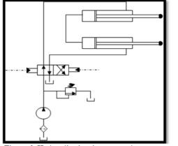
Figure 3: Hydraulic circuit commands concrete cylinders
