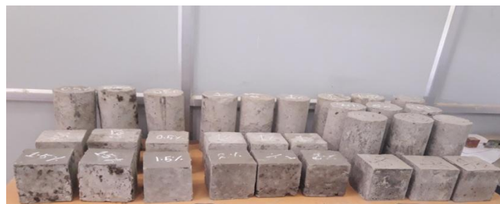
Fig.2. Cube and cylinder specimens ready for test
