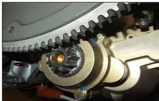
Fig 1: Assembly of Flywheel ring gear and Starter pinion gear
