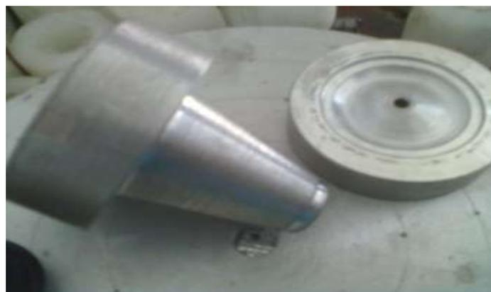
Figure 8. Nozzle with Top Plate
