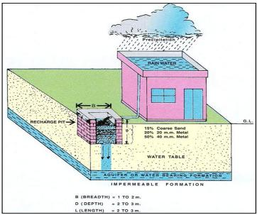
Figure 4: Schematization of roof-top rainwater harvesting through recharge pit [7]
