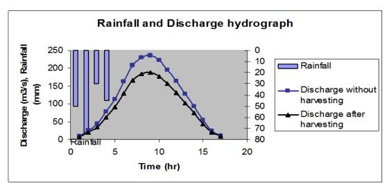
Figure 5: Rainfall chat and discharge hydrograph for 200 mm rain in one
