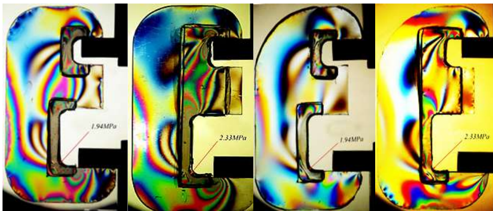
Fig 8: a) Model "OC" Fig 8: b) Model "OE" Fig 8: c) Model "RC" Fig 8: d) Model "RE"
