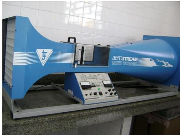
**Figure 2** - Wind tunnel used for determining the drag coefficient.
