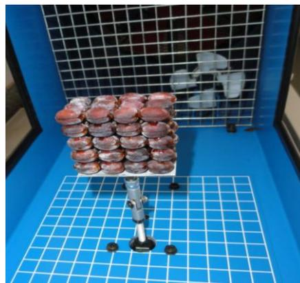
**Figure 4** - Coffee fruit cluster in wind tunnel test section.
