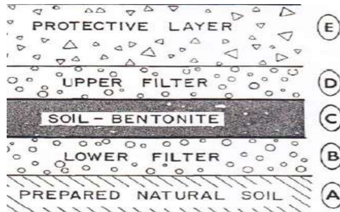
Fig.1. A typical cross section area of soil-bentonite landfill liner (Chapius 1990)
