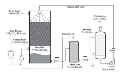
To increase the absorption of  $CO_2$  and  $H_2S$ , biogasis usually compressed to 900–1200 kPa and a high surface area packing mediais used. Inside the scrubber, biogas flows counter- currently (opposite direction) towater that is sprayed from the top of scrubber, and the cleaned biogas can contain 96%  $CH_4$  after drying.
