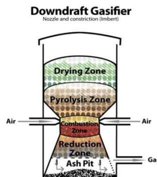
Fig.1. Working Principle of an Imbert type Downdraft Gasifier
