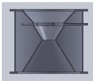
The other components include a hopper section, ash section and flanges.
