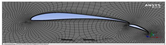
Fig 2 Airfoil S1223 With 1 Element
