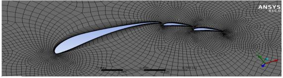
Fig 3 Airfoil S1223 With 2 Elements
