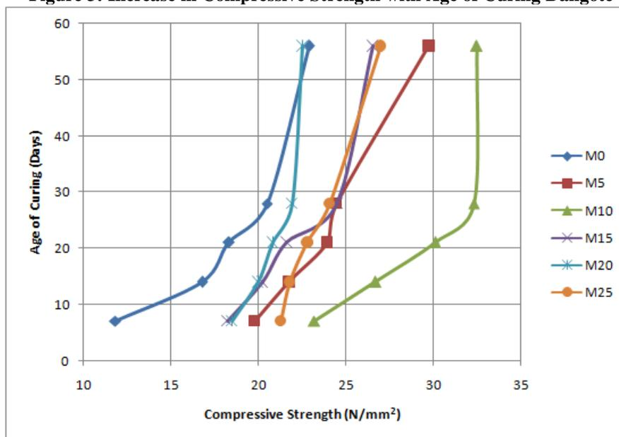
**Figure 4: Increase in Compressive Strength with Age of Curing Ibeto**
