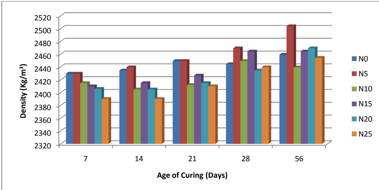
Figure 6: Density Result for all days of curing with Dangote Cement
