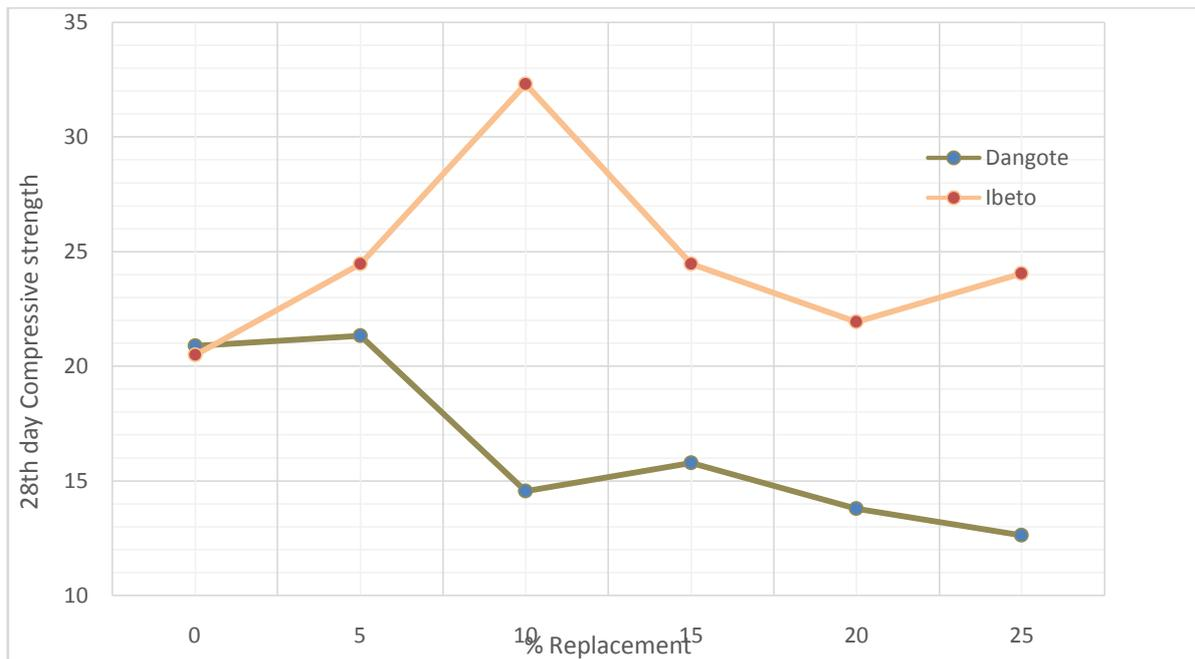
**Figure 5; Variation in Compressive Strength of the Concretes at 28<sup>th</sup> Day of Curing**
