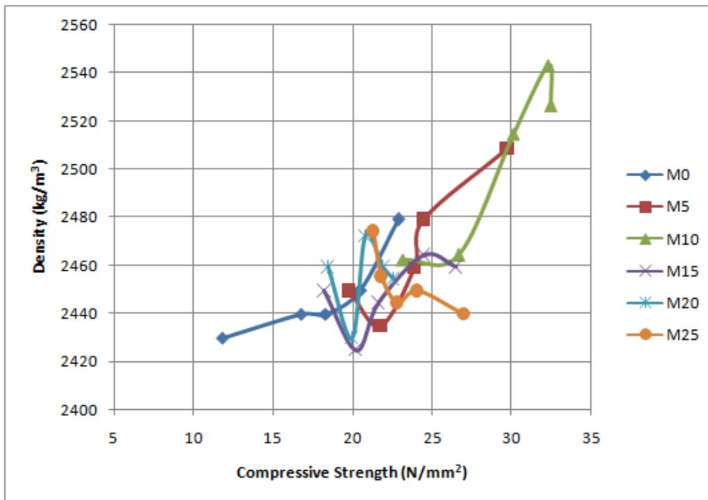
Figure 9: Variation of Compressive Strength with Density with Ibeto Cement
