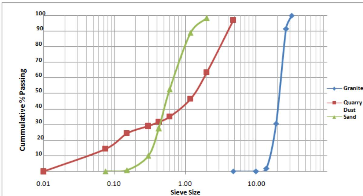
Figure 1: Particle Size Distribution for Gravel, Sand and Quarry Dust.
