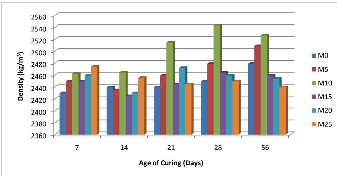
Figure 7: Density Result for all Days of Curing with Ibeto Cement
