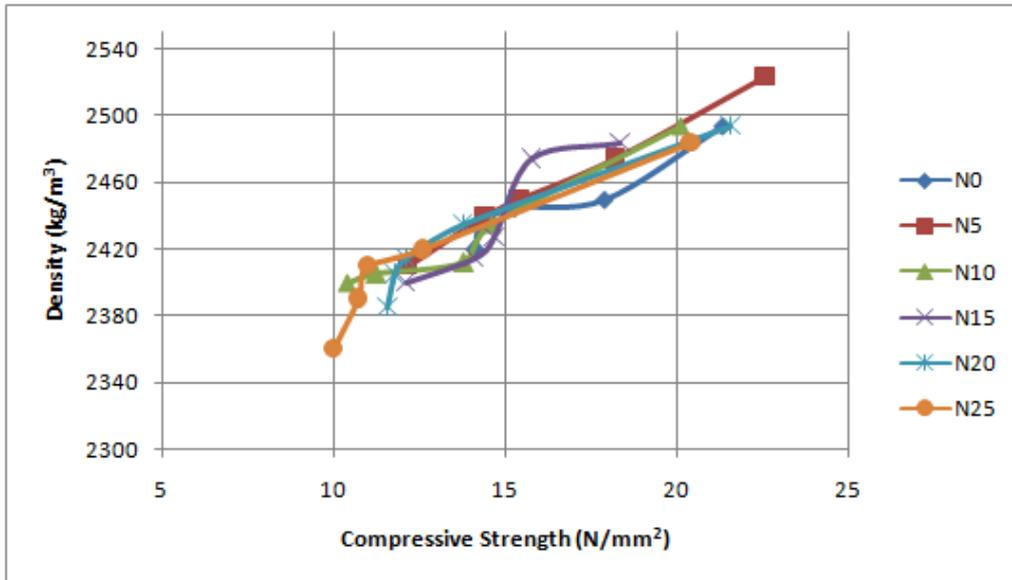
Figure 8: Variation of Compressive Strength with Density with Dangote Cement
