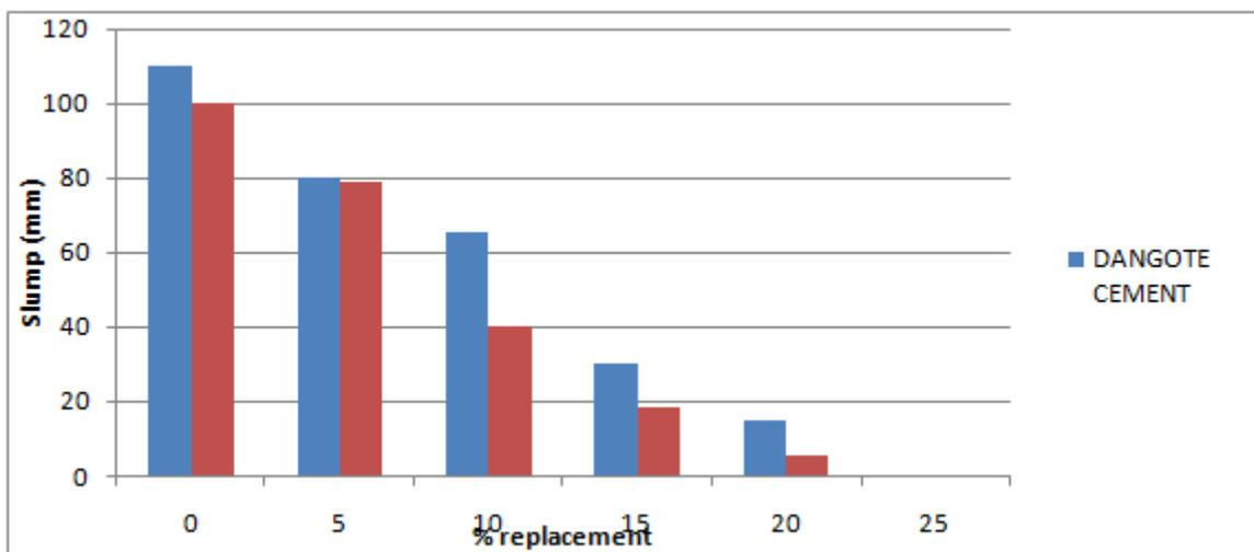
**Figure 2: Workability of the Concrete mixes with the Two Portland Cement brands**
