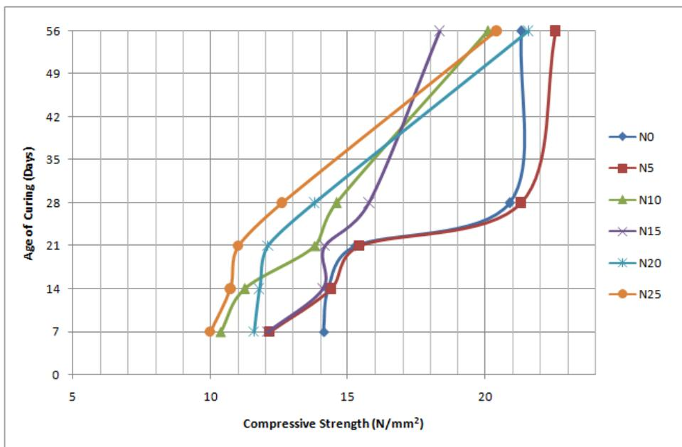
**Figure 3: Increase in Compressive Strength with Age of Curing Dangote**
