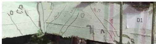
Fig (18) Crack pattern of beam (D1)
