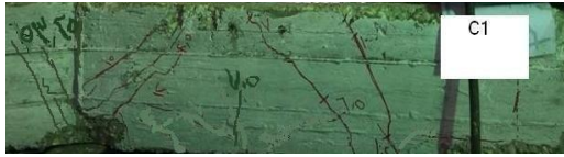
Fig (16) Crack pattern of beam (C1)
