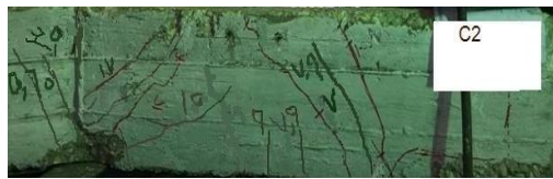
Fig (17) Crack pattern of beam (C2)
