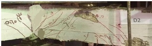
Fig (19) Crack pattern of beam (D2)
