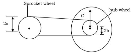
When the pedals and sprocket wheels complete a revolution, the hub wheel rotates through  $\frac{2\pi a}{2\pi b}$  revolutions,
