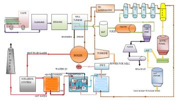
Fig.1.2 Raw Sugar Milling with Proposed Cooling System
