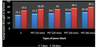
Fig .No.7. Compressive strength of paver block at 0.4% fiber by changing top layer thickness
