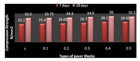
Fig .No.4. Compressive strength at 7 & 28 days for Paver blocks without and with fibers
