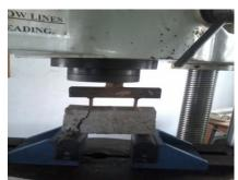
Fig .No.3. Flexural strength test
