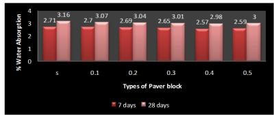
Fig .No.5. Water absorption at 7 & 28 days for Paver blocks without and with fibers
