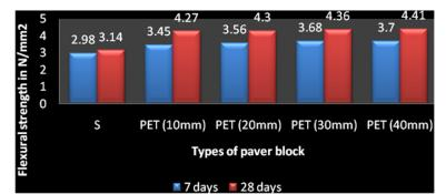
Fig .No.8. Flexural strength of paver block at 0.4% fiber by changing top layer thickness
