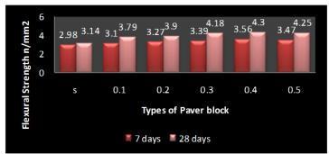
Fig .No.6. Flexural strength at 7 & 28 days for Paver blocks without and with fibers
