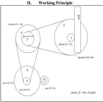
Fig. 1. Schematic diagram of gear mechanism.
